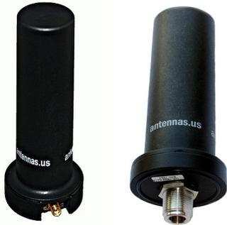
For embedded and weight sensitive applications, such as self-buoyant air and water platforms, like balloons and buoys, we offer a 30 gram (1 oz) lightweight version: UL-1624-341R-LIGHT (select from above Base/Flange drop down menu). It is enclosed in a light housing, measuring 27.5 mm (1.08") OD x 99 mm (3.9") L, with an SMA Female connector at its bottom center.
